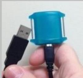
Figure 1: Triaxial accelerometer
